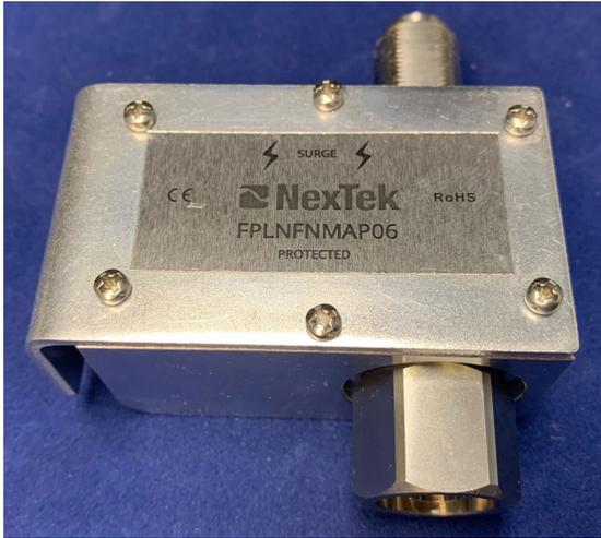
**RF DC Pass Fine Protector, 400-2700 MHz, Type N, Bulkhead, 6VDC, 25kA** - The FPL series is a RF broadband device designed for surge and lightning protection applications where DC Pass is required to power the electronics. The FPL unit offers excellent surge / lightning suppression for distributed antenna systems (DAS), Tower Top amplifiers, GPS applications requiring a DC Pass design. The FPL series demonstrates excellent RF characteristics while offering outstanding surge protection.
